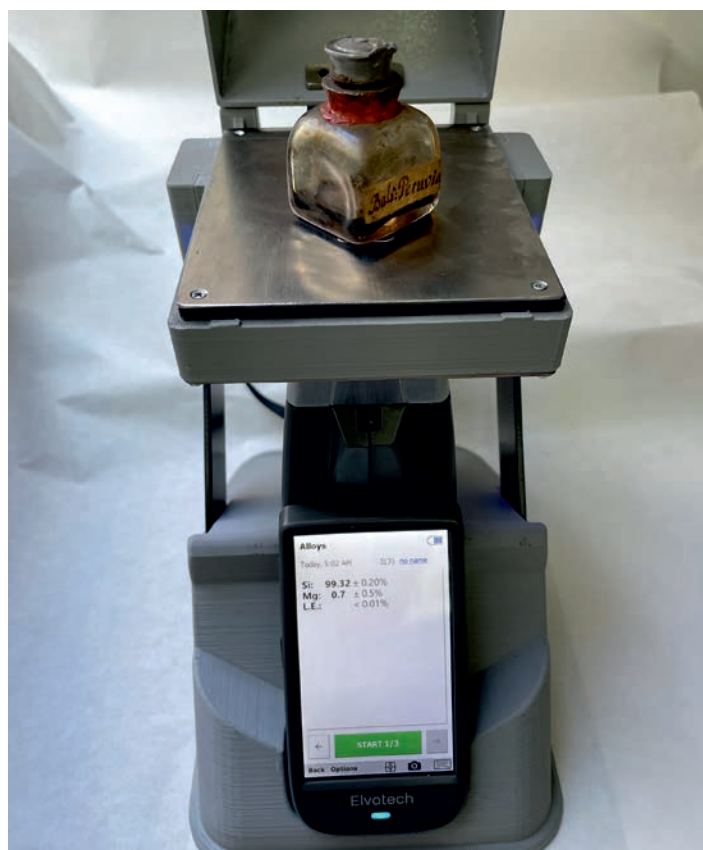
Fig. 4. XRF (X-ray fluorescence) test showing the composition of the glass of an apothecary container (Colecția MNIT, no. IF 1948, image from the MNIT Archive).
